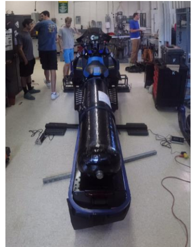
Figure 8: Setup to Measure the CG
